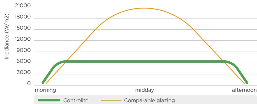
Controlite® blocks 80% of solar heat gain (W/m²).
